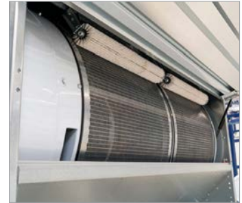
Cleaning brushes are mounted on a spring-loaded arm for efficient even load on the outer screens.
